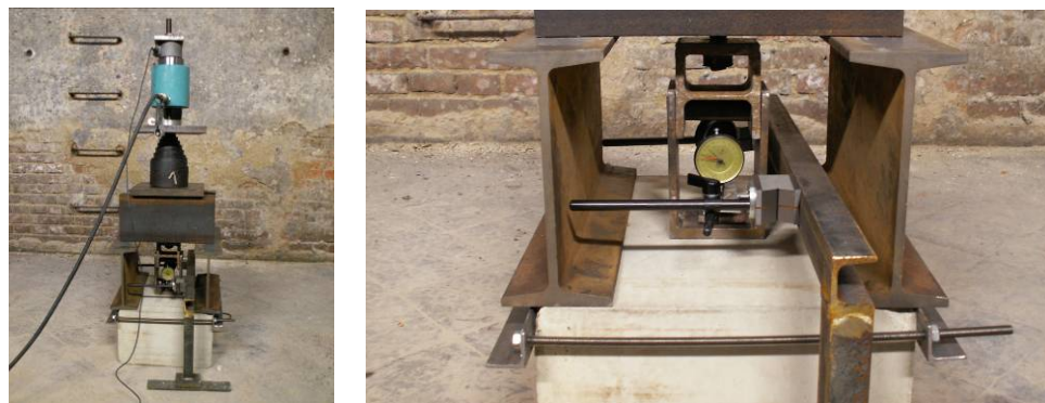
Fig. 5. Experiment with long-term loading of steel bonded anchors
